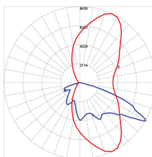
EANB Type II - Asymmetric Narrow (F2) 14,400 Lumens, 5000K (EANB_F2750__IES)
