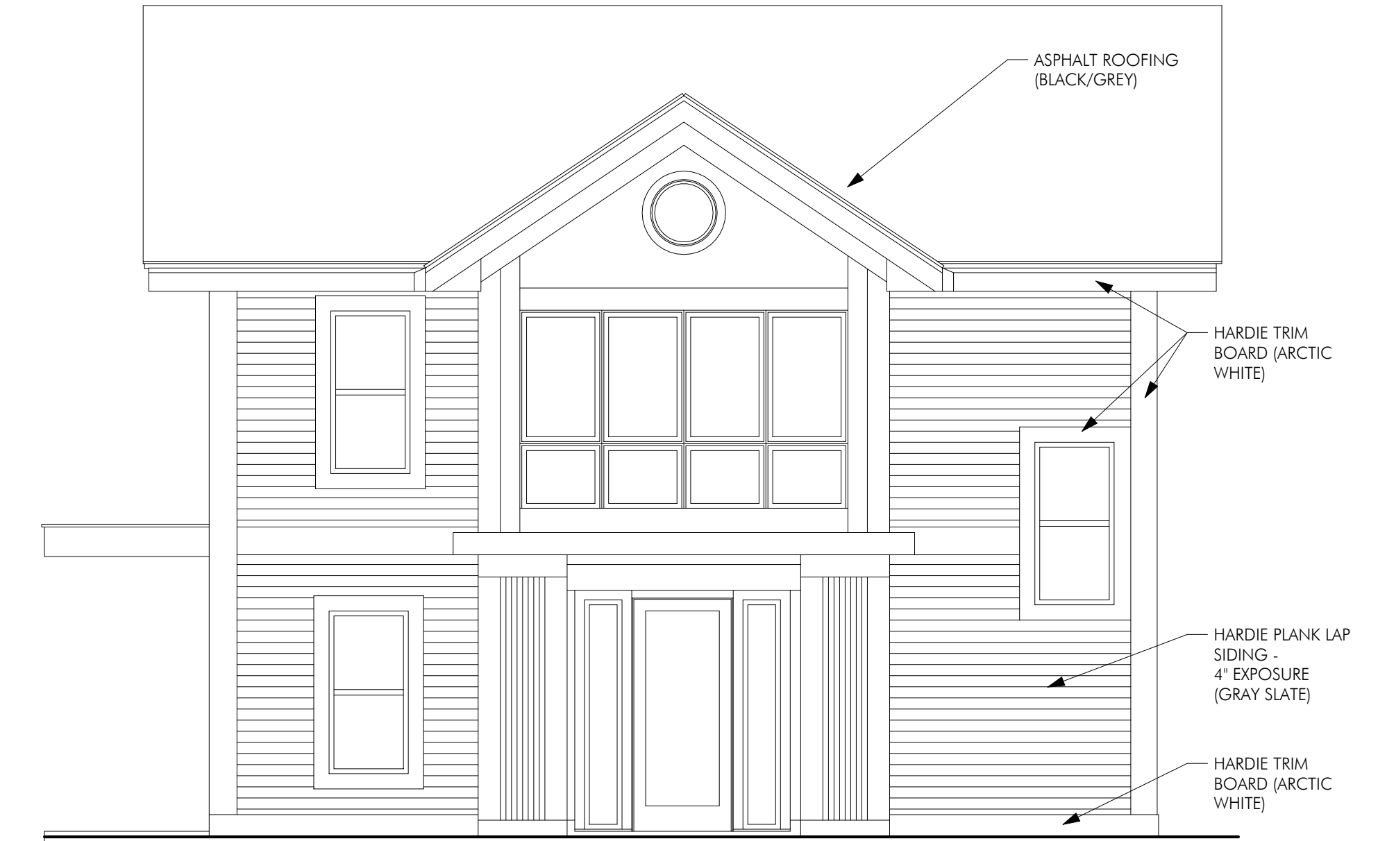
2 | CHASKA YARDS - Unit 1 - WEST ELEVATION A251 | 1/4" = 1'-0"
