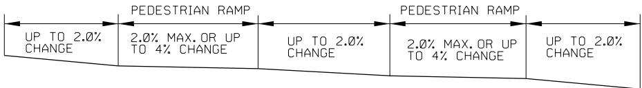
FLOW LINE PROFILE "TABLE" - TWIN PERPENDICULARS
