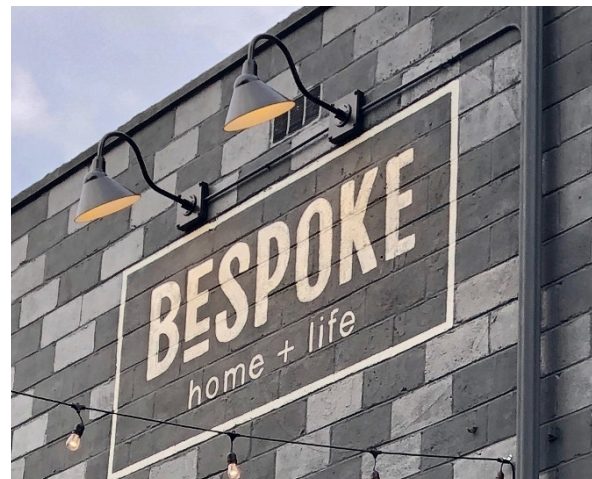
Example of gooseneck fixtures illuminating an entrance sign at the rear of a building, along with string lights. (Collingswood, NJ)
