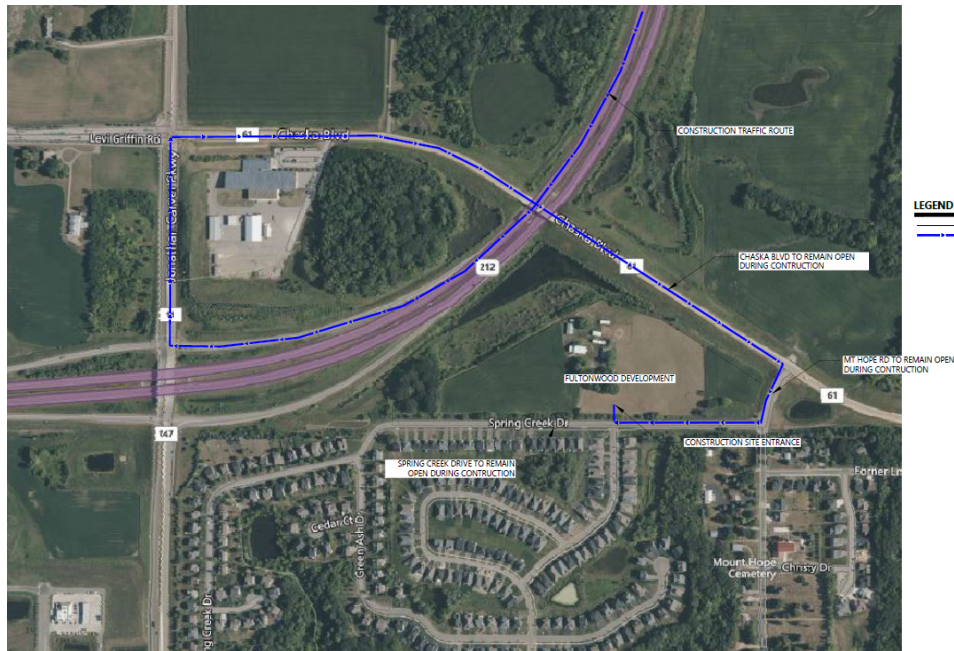
Figure 9: Construction traffic plan
