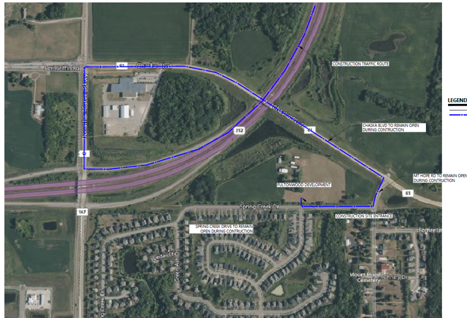
Figure 9: Construction traffic plan
