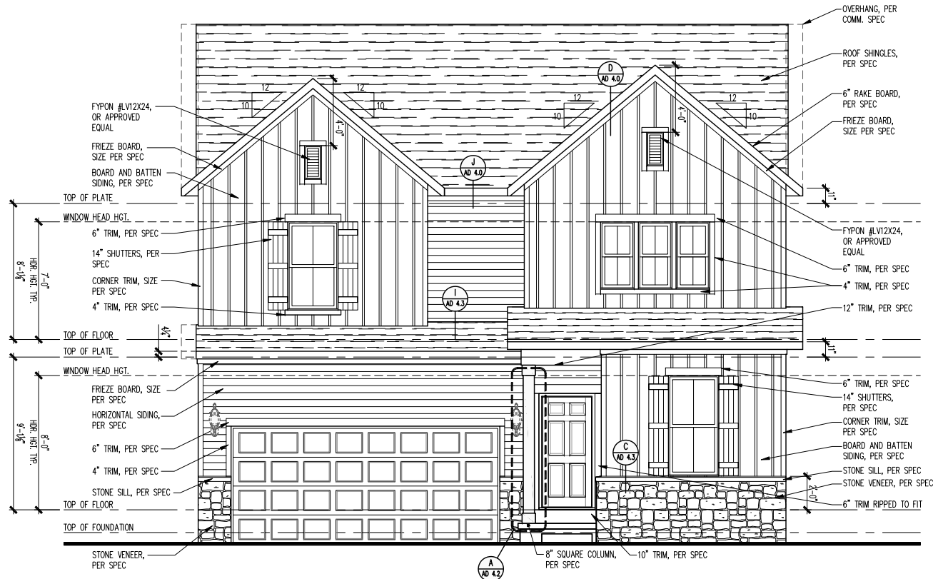
FRONT ELEVATION - FH201 SCALE: 1/4" = 1'-0"
