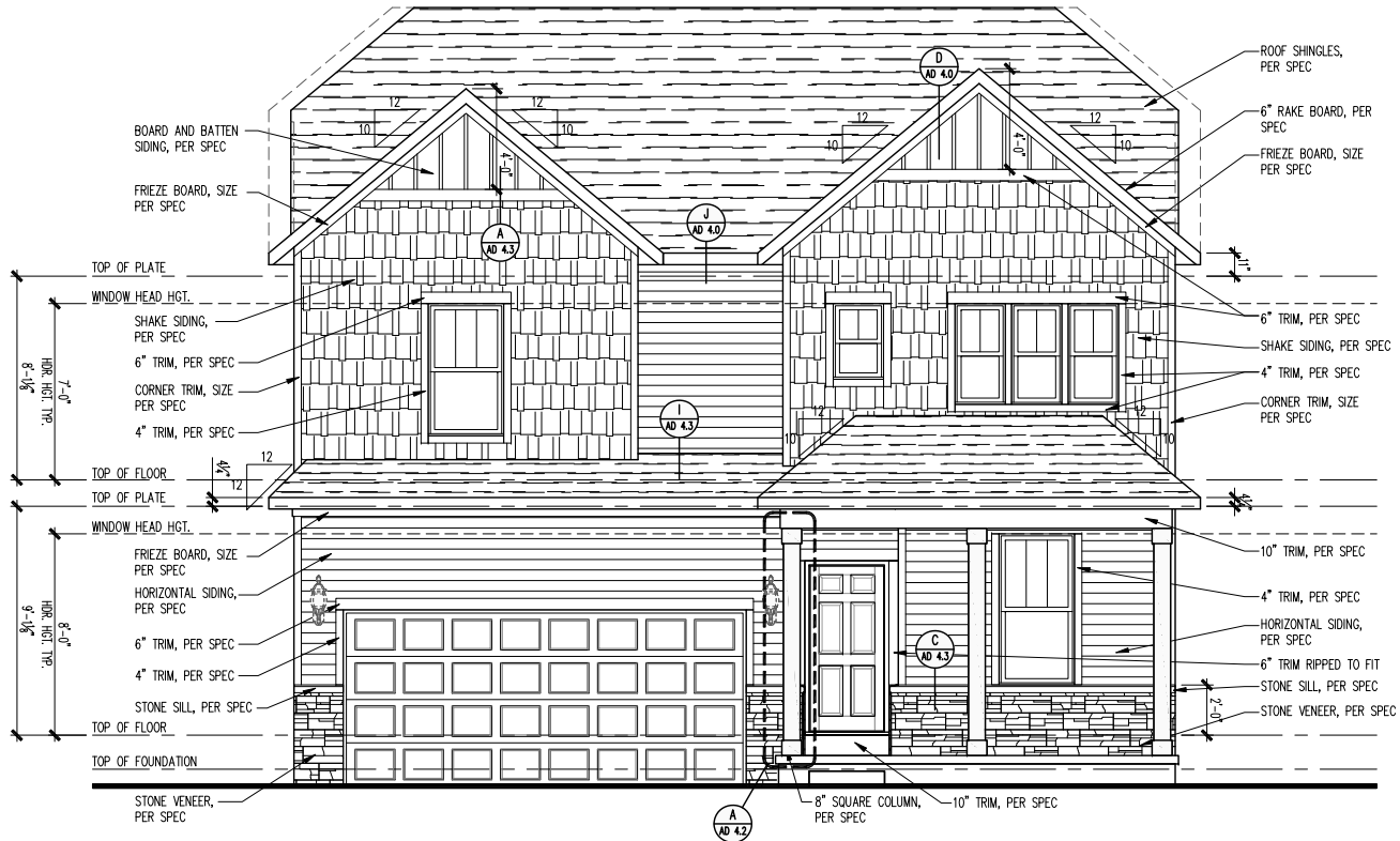
FRONT ELEVATION - NC201 SCALE: 1/4" = 1'-0"
