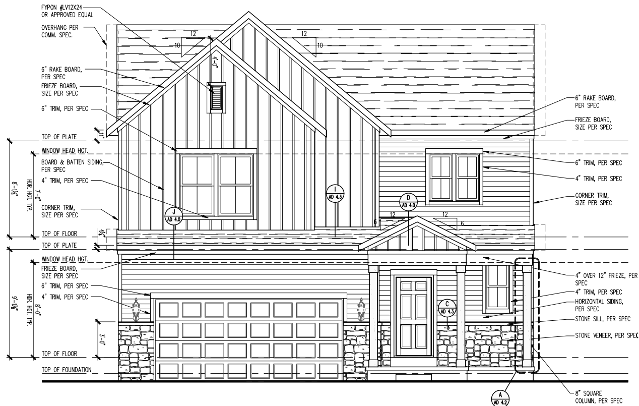
FRONT ELEVATION - FH201 SCALE: 1/4" = 1'-0"
