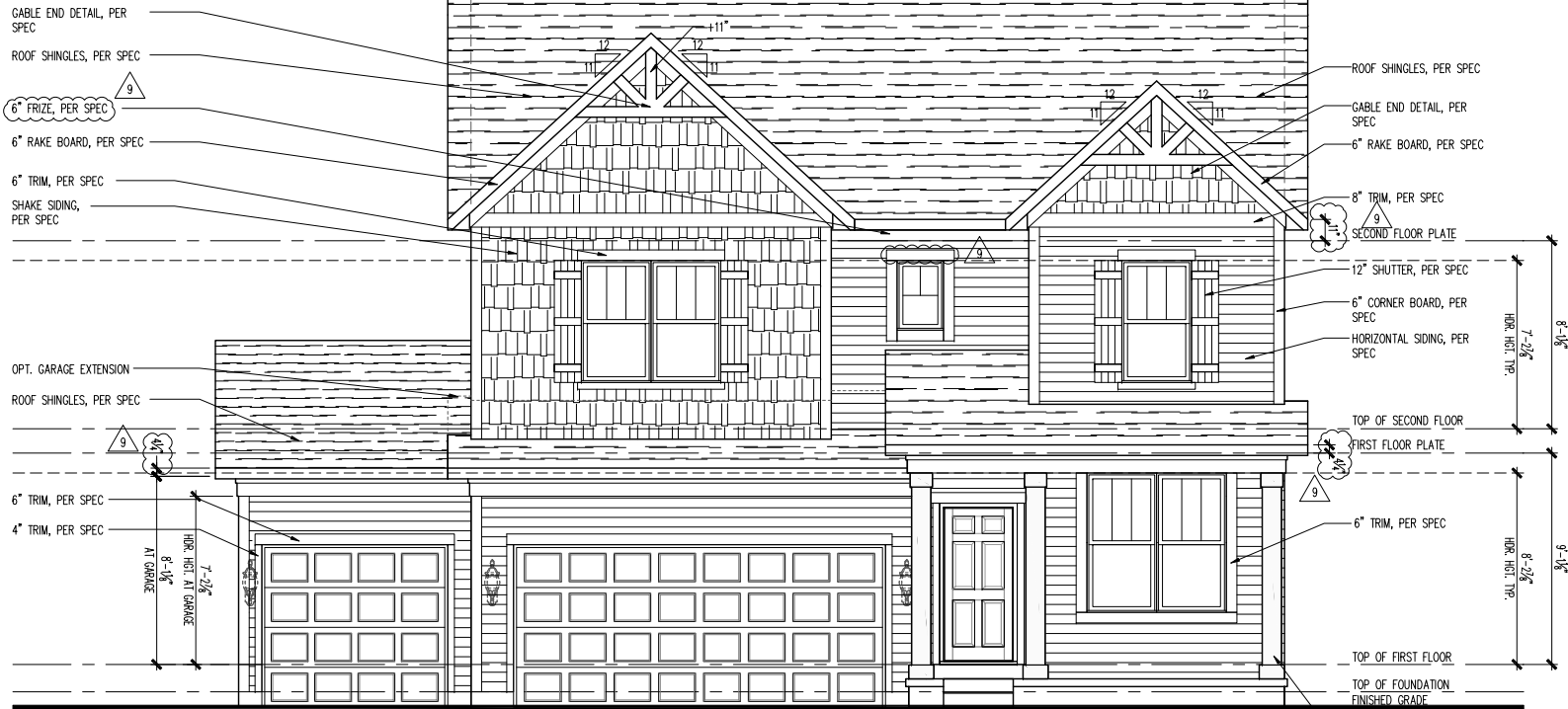
FRONT ELEVATION SCALE: 1/4" = 1'-0"
