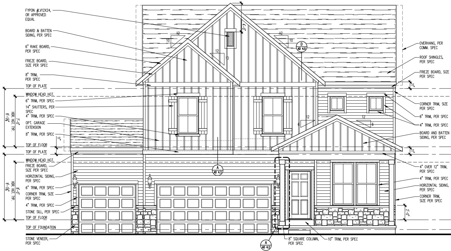
FRONT ELEVATION - FH201 SCALE: 1/4" = 1'-0"
