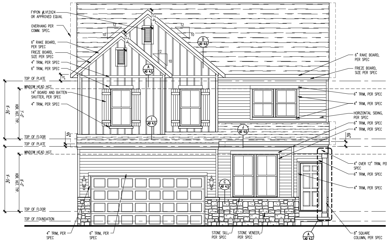
FRONT ELEVATION - FH201 SCALE: 1/4" = 1'-0"
