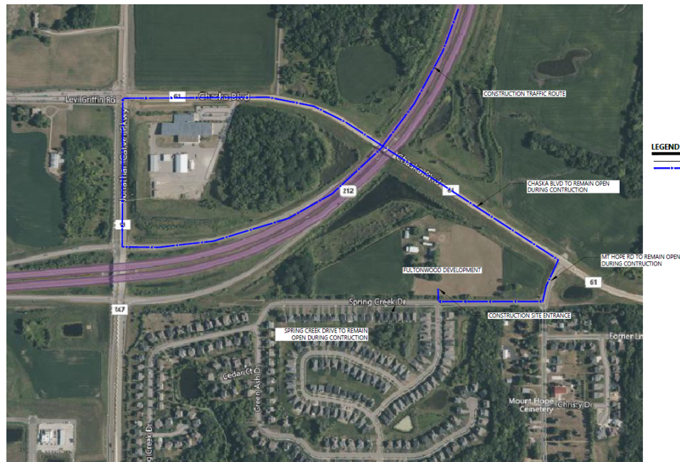
Figure 10: Construction traffic plan
