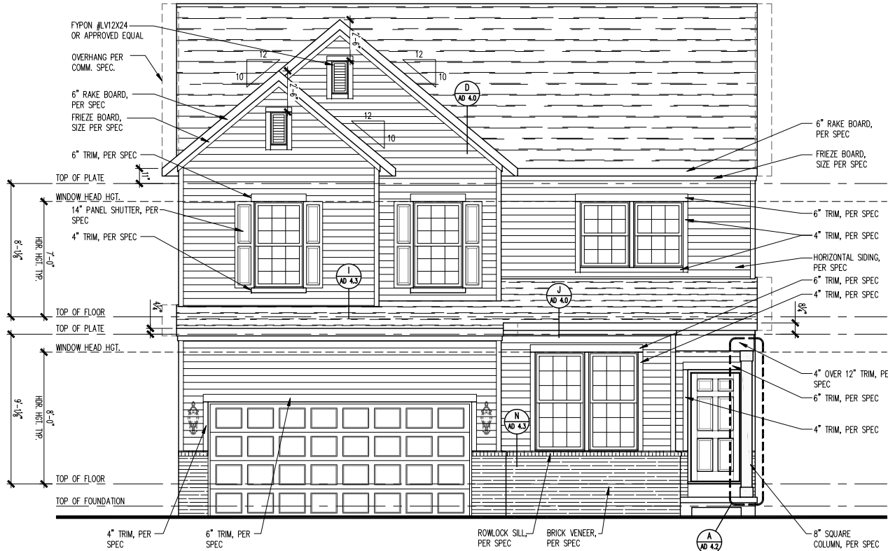
FRONT ELEVATION - HR201 SCALE: 1/4" = 1'-0"
