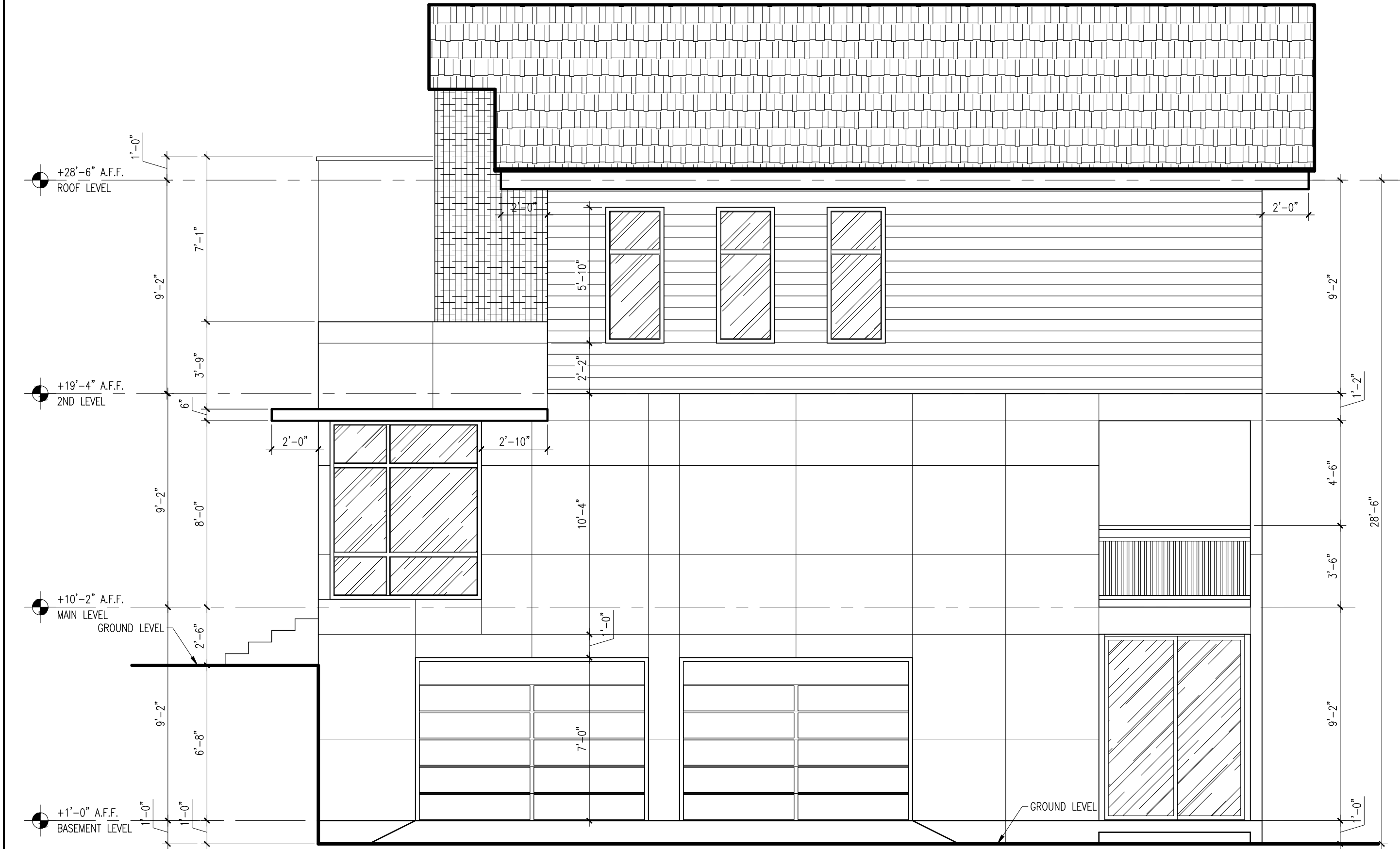
ARCHITECTURAL RIGHT ELEVATION
