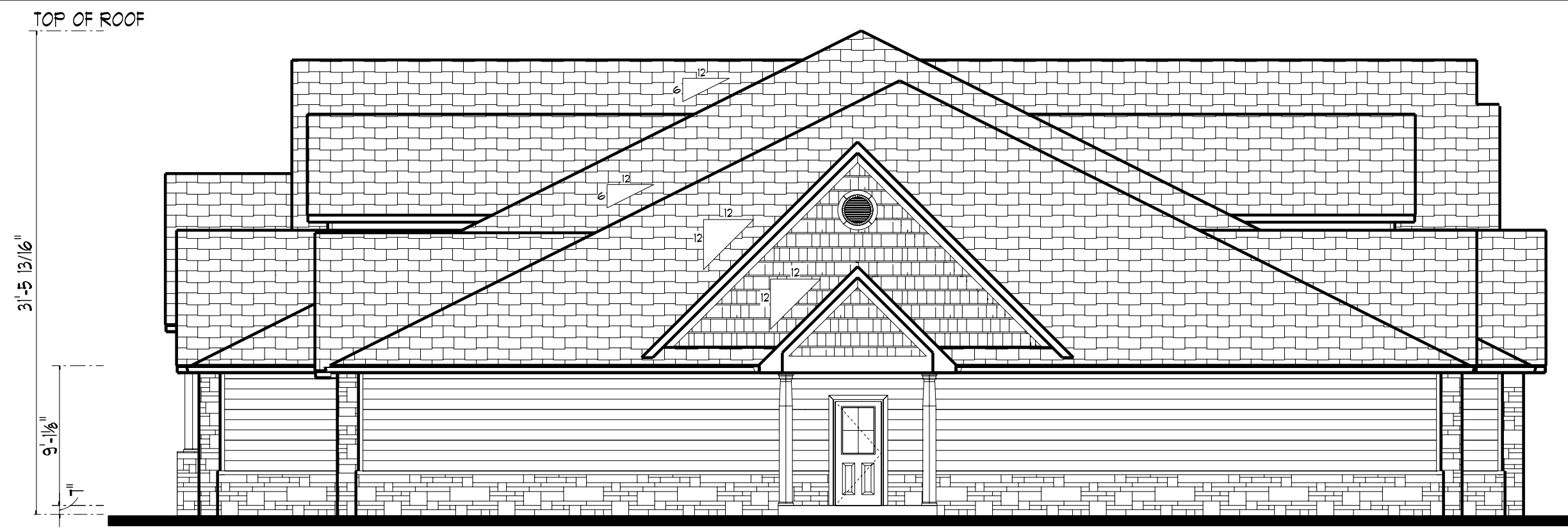
3 EAST ELEVATION (RIGHT SIDE OF BUILDING)
