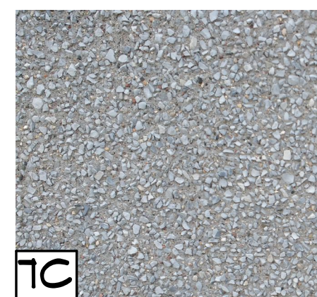
7C RAISED AGGREGATE CONCRETE COLOR MATCH "KING'S GREY"
